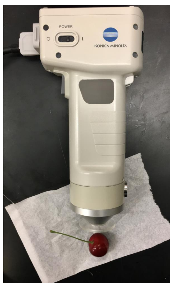
Figure 3: Colorimeter used to measure L* a* b* values
