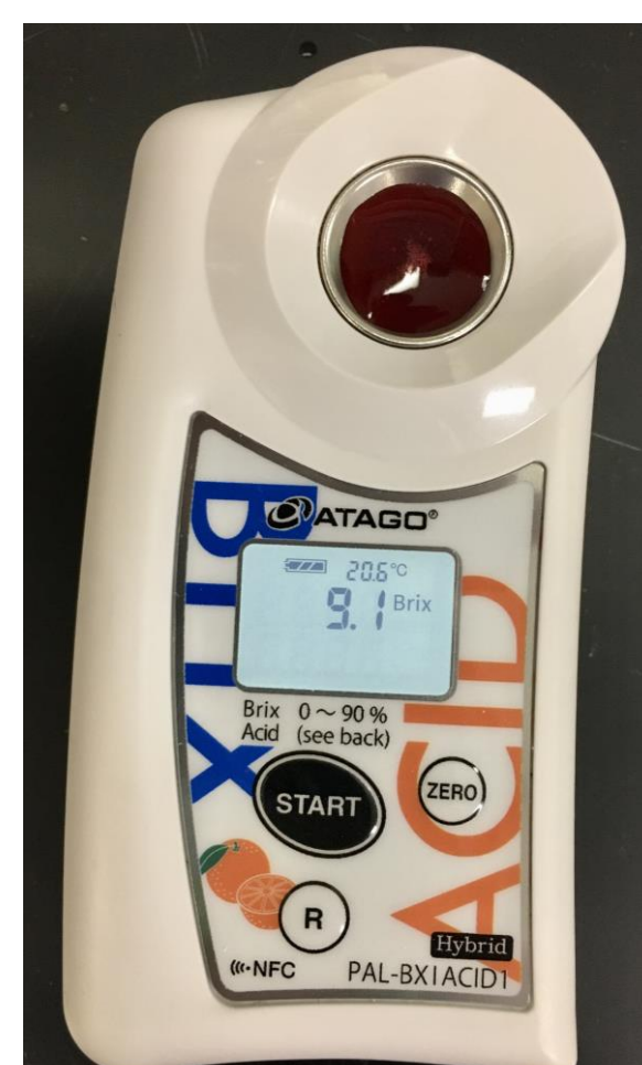
Figure 4: Refractometer used to measure Brix (sugar percentage) on juice samples
